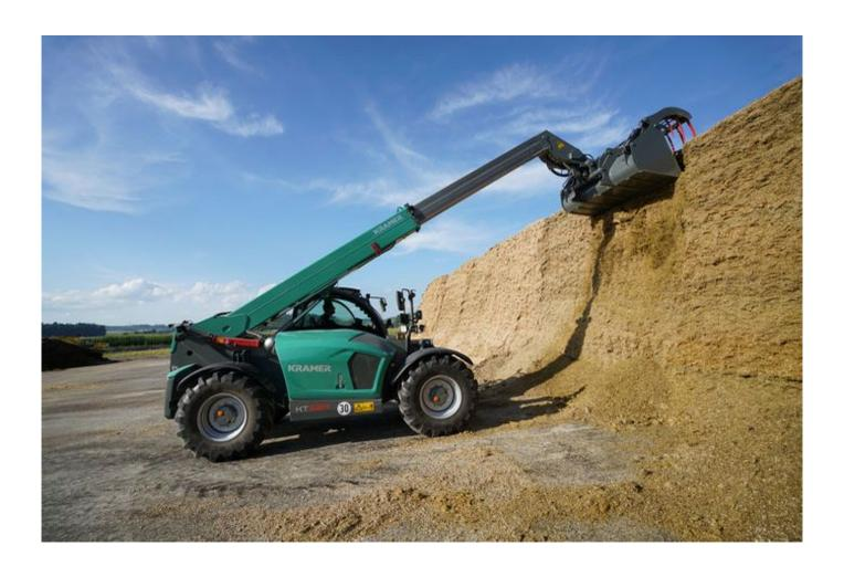
The top model KT559 has a lift capacity of 5.5 tonnes and a stacking height of 8.75 metres. The 156 hp Deutz engine with a torque of 609 Nm combined with a max. bucket volume of up to 4  $\rm m^3$  allows for maximum handling capacity for applications in professional agriculture. The sensitive load sensing gear pump conveys up to 187 l/min, thus offering enough power for quick work cycles. Trailer loads of up to 20 tonnes are also no problem for this telehandler.
